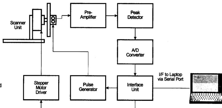
**Schematic diagram of the data capture system. The computer program controls the position of the stepper motor and sends out ultrasound pulses in known directions. The echo signal is recorded for each ultrasonic pulse and used to build up an image of the cave walls.**
