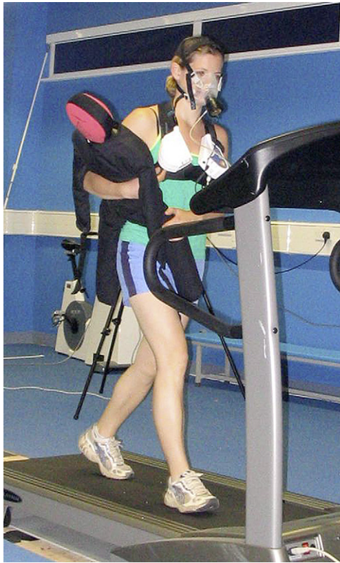
Fig. 1. Participant walking on treadmill wearing Metamax unit and carrying mannequin.
